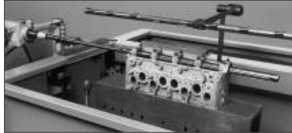
Cylinder head being honed on CH-100 Honing Machine with a hand fed Porta-Hone.
